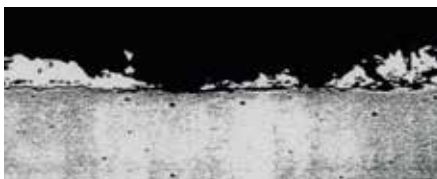
Microscopic picture view of galvanized steel after weathering
