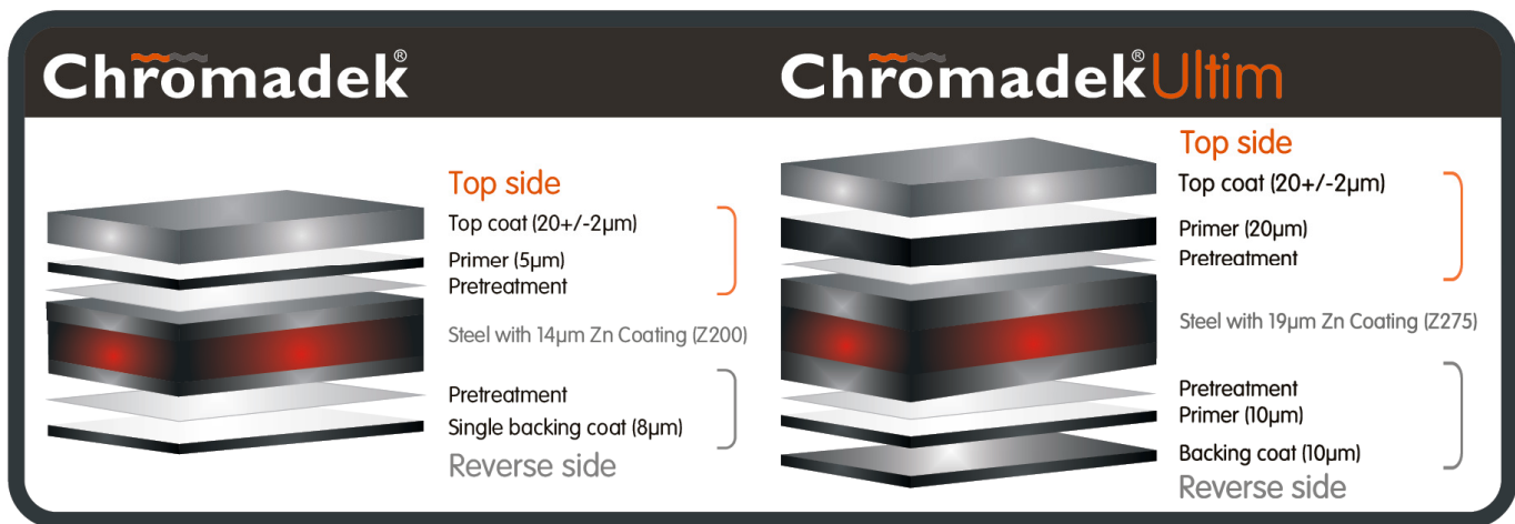
Figure 1: Coating structure of Chromadek® Standard and Chromadek Ultim®.
