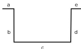
Box Gutter with Double Outfolds
