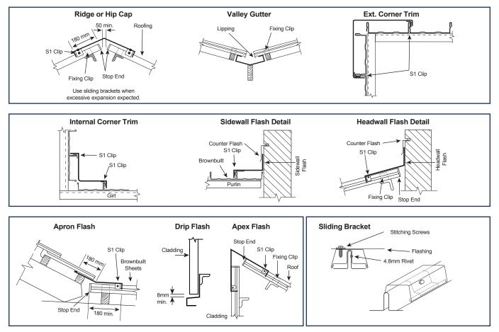
\* When sheet lengths are over 30m (20m for Aluminium) flashings must be fixed to sheets using sliding brackets.
