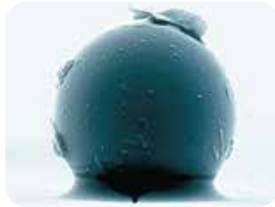
Figure D Microscopic picture shows dirt bonding to the surface of conventional pre-painted steel.
