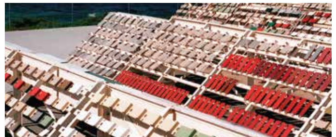
Figure 2: Test panels placed at BlueScope exposure rack
