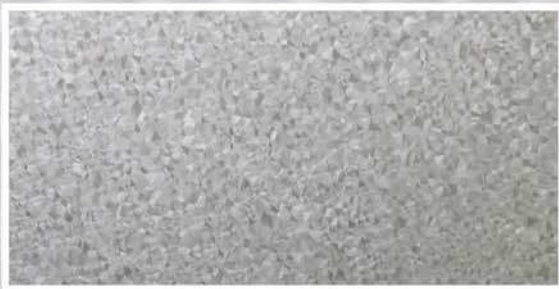
Photographic Representation of ZincAL® Spangle
